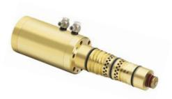
2/2-way valve air operatedpressure range PN 0-500 barorifice DN 15 mmdesign cartridgefunction valve
